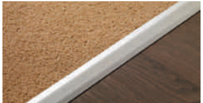
Profile B - L2.7m x W38mm Laminate to Carpet or Linoleum Suitable for use from laminate to carpet or linoleum, this profile will also bridge differences in height of between 4mm to 15mm Aluminium SDH0942
